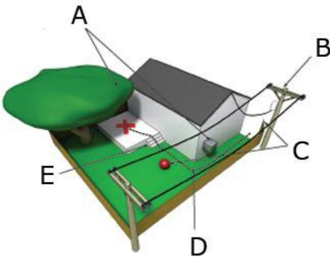
**A** - Obstacles such as overhanging tree limbs, awnings, protruding gas meters, water meters, and A/C units can prevent easy access.
