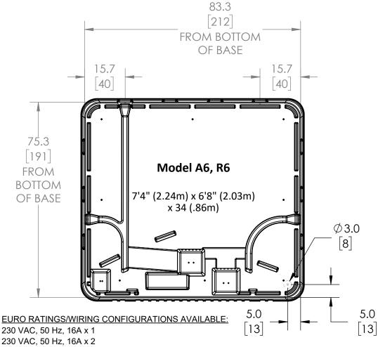
230 VAC, 50 Hz, 32 A 400 VAC, 50 Hz, 16 A x 3 (3 ph
