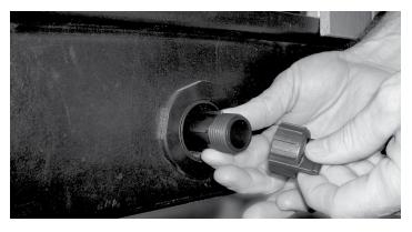
**NOTE:** Drain is fully extended at approximately 2 inches (5 centimeters).
