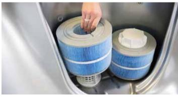
**Step 4:** Using a garden hose with a nozzle or other highpressure device, clean cartridge(s). Work first from the inside, top to bottom on each pleat then from the outside, top to bottom on
