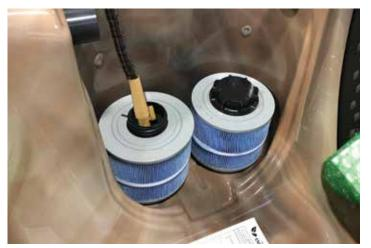
**Step 4:** Fill to the water level indication on the faceplate of the filter assembly.
